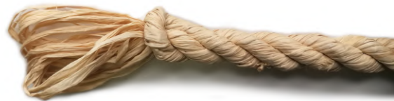
3-ply rope with the typical turn of the strands locking the third strand
