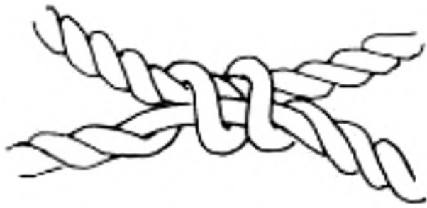
Illustration of 2-ply net from Hedeby 143 and Bryggen 144
